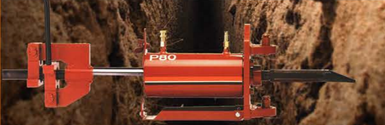
40 Tons For Pipes up to 15cm
